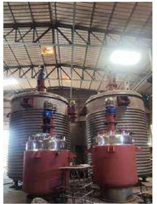
All LVE Pressure Vessels and Reactors are designed and fabricated in strict accordance with ASME (Section VIII, Division I). ASME vessels can be fabricated from Carbon Steel, Stainless Steel or Nickel Alloy materials.
